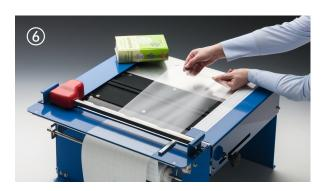
Pull the film off the roll to the measured coloured spot.
